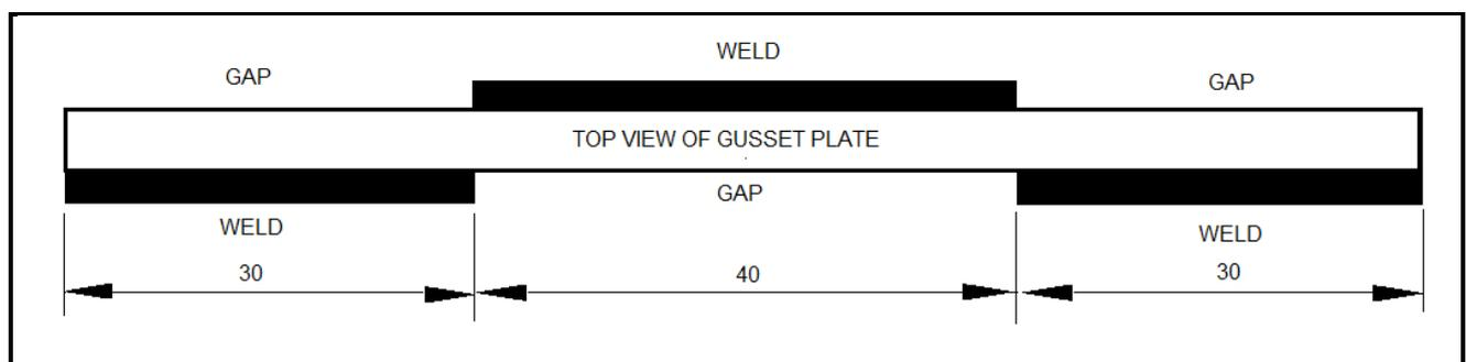
FIGURE 3: Top view of welding on gusset plate
