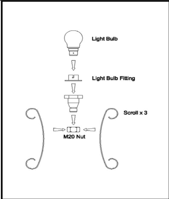
FIGURE 5: Exploded view Lamp stand
